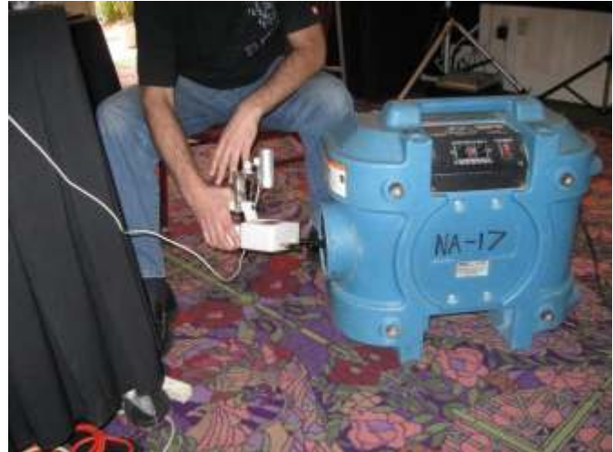
A seminar attendee uses a hand-held particle meter to apply the PHEAF standard procedures to a high efficiency collection device.
